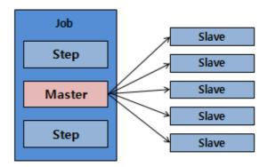
Note that the Job progresses from left to right as defined in the foregoing figure. One of those steps is defined as the master label and the slave labels are identified as the instances of Step whose results are reverted to the master. Being a typical form of remote service, slave is transmitted to the local thread. In Spring, it is guaranteed that, in metadata of JobRepository, each slave is executed once for each job.
